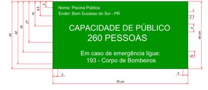
PLACA M-2 Conforme Figura 2 - Da NPT 20.
